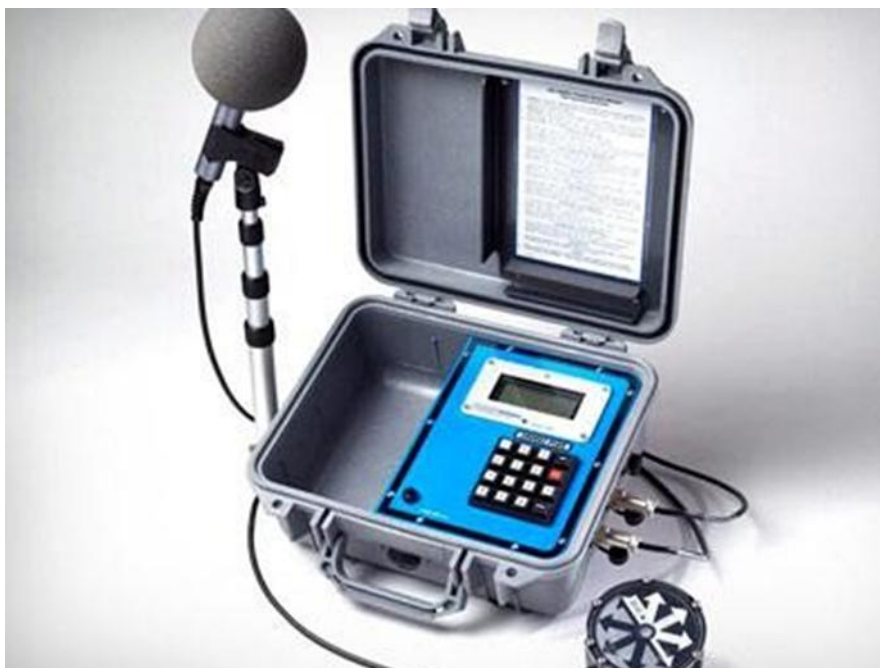
Figure 3.1-4: Vibration monitoring equipment
