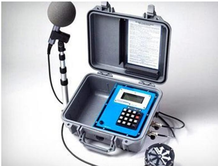
Figure 3.1-4: Vibration monitoring equipment
