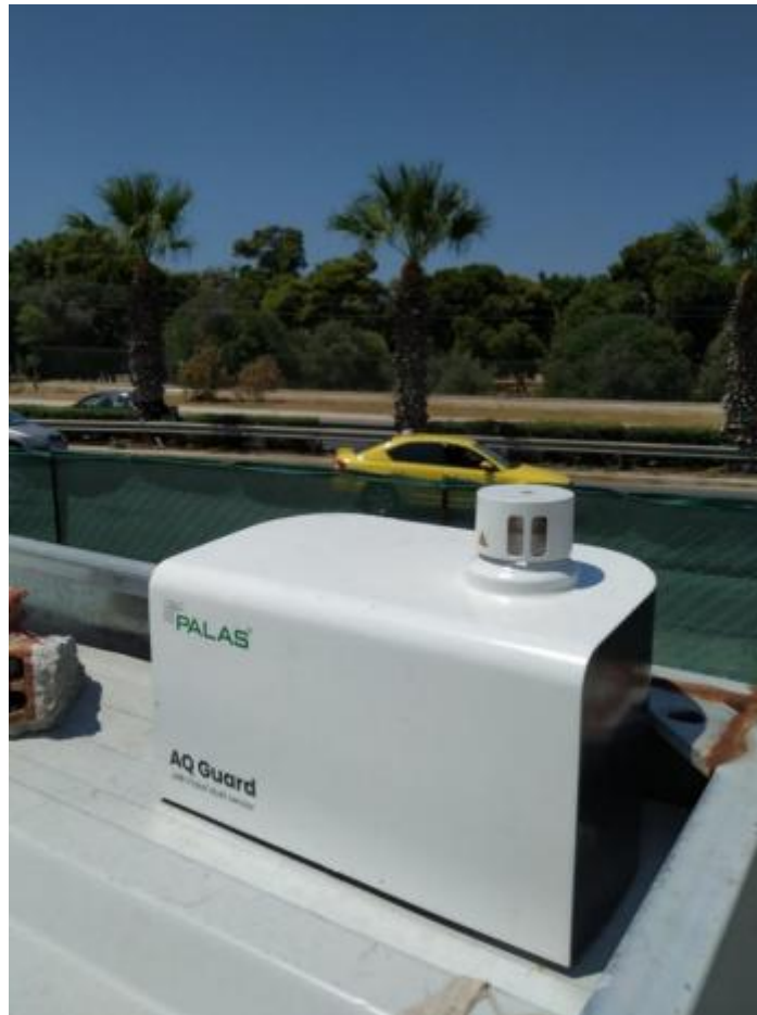
Figure 2.2-1: AQ Guard ambient analyzer from German manufacturing company of Palas for the measurement of fine particulate matters
